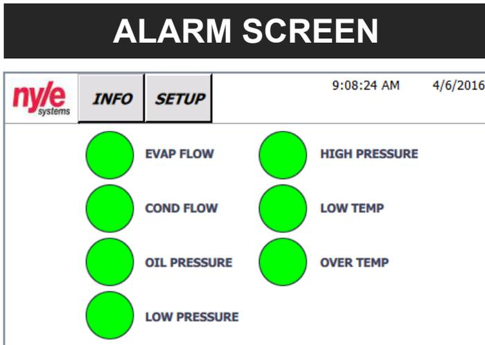
“**LOW TEMP**”: GREEN indicates that the water temperature leaving the evaporator is above the shutoff value. RED indicates that the water temperature leaving the evaporator is below the shutoff value.
