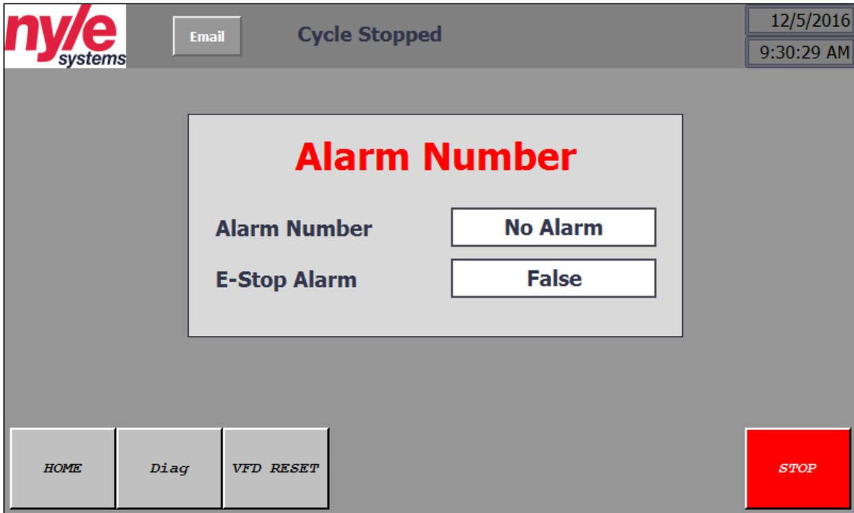
The alarm screen allows the user to view currently active alarm conditions. The alarm number will correspond with a code produced by the blower VFD and found in the VFD manual.
