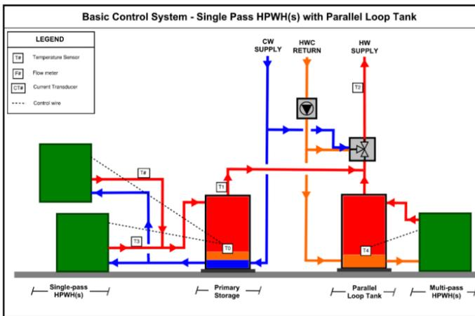
**Figure 5. Parallel Loop Tank Configuration**
