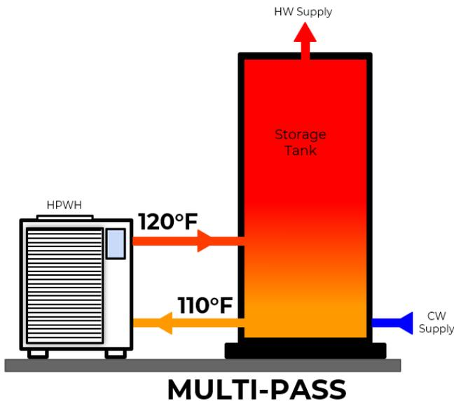
Heats water to working temp. in multiple passes
