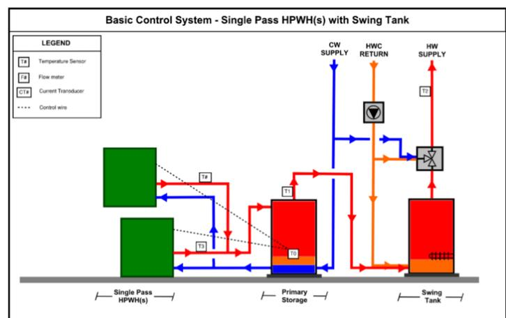
**Figure 4. Swing Tank Configuration**
