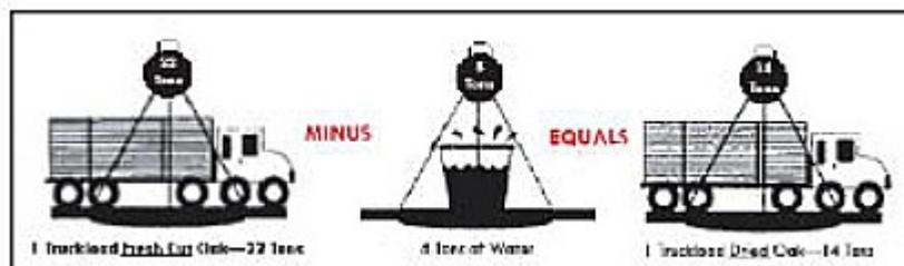
of 8,000 board feet weighs about 43,560 pounds—just under 22 tons. Once you remove enough water to get the oak down to a moisture content of 6%-8%, it weighs about 3.5 pounds per board foot. So that truckload now weighs 28,000 pounds, or about 14 tons. That means that to completely dry a truckload of 8,000 board feet of oak, you have to remove 15,560 pounds of water—almost eight tons! That's why choosing the right drying system and using the proper method are so important.
