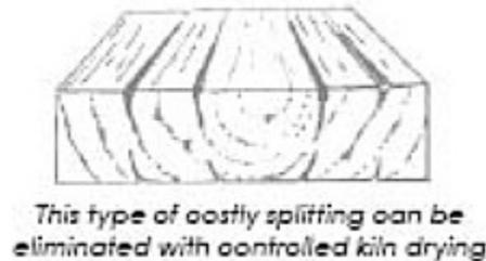
Controlled drying in a kiln, especially when drying from the green state, reduces or eliminates splitting and checking. When lumber is air dried, however, there is no control over the drying process, and the weather can easily cause splitting and checking that results in losses.
