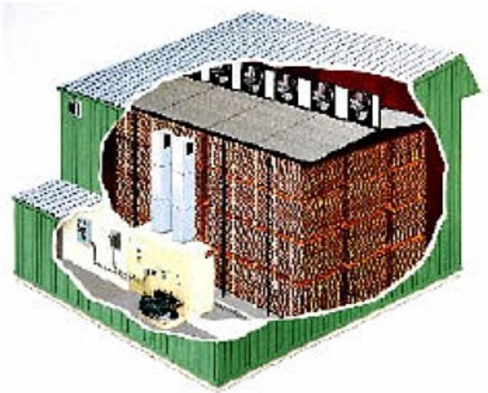
Drying in a closed kiln chamber, shown here, allows accurate control over critical drying conditions such as airflow, temperature, and humidity.
